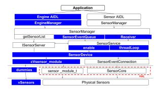
Fig. 2: SOUL's implementation in Android. The colored boxes indicate SOUL's modules added to Android.
