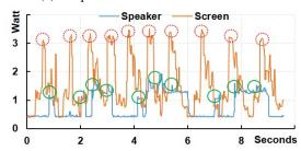
(b) The speaking and screen consume 22.14 and 40.94 mWH, respectively. Each circle shows the moment that a user acknowledges the current time.
